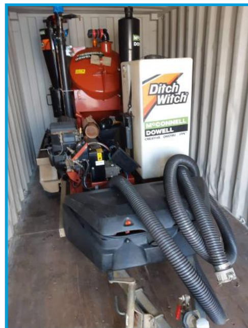
Above: Ditch Witch vacuum excavator in shipping container
